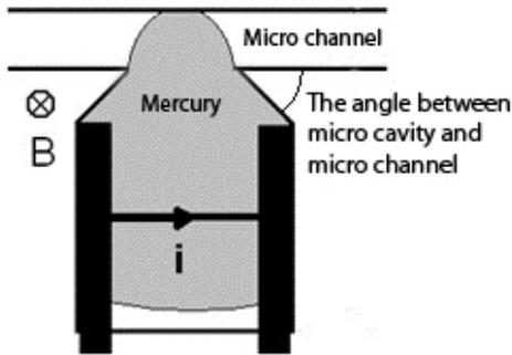
Fig. 1 Schematic view of the micro cavity – micro channel angle
